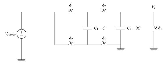
In the first phase, all of the switches labeled  $\phi_1$  will be closed and all switches labeled  $\phi_2$  will be open. In the second phase, all switches labeled  $\phi_1$  open and all switches labeled  $\phi_2$  close.
