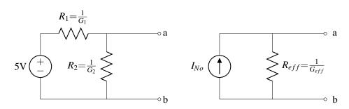
(e) The second step, using the Norton equivalent circuit you found in part (d), what is the range of  $G_{eff}$  that achieves  $3.80V \le V_{out} \le 4.20V$  in terms of  $I_{No}$  and  $G_l$ ?
