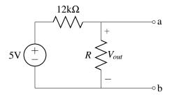
(b) Now consider loading the circuit with a resistor of  $1k\Omega$  as depicted in the following circuit with the same value of the resistor *R* as calculated in part (a). What is the voltage  $V_{out}$  now?
