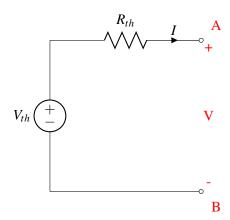
Now how would you figure out  $V_{th}$  and  $R_{th}$  for the Thevenin equivalent circuit? If we plot the I v.s. V relationship where V is the voltage drop from A to B and I is the current flowing into A (as shown in the figure), we would get a graph that looks like the following.
