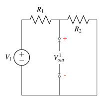
We know that  $V_{out}^1 = \frac{R_2}{R_1 + R_2} V_1$ . Next we compute the output voltage due to and hence source  $V_1$  will be replaced with a short circuit.
