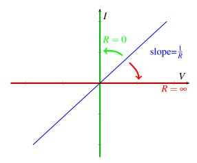
We know that the slope of the line is equal to  $\frac{1}{R}$ . What happens when R becomes infinite? Then the line becomes the x-axis, which corresponds to an open circuit as we've seen earlier. Now what happens when R is zero? The line becomes the y-axis, which corresponds to a short circuit.
