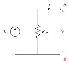
We call the first circuit containing a voltage source and a resistor the **Thevenin equivalent circuit**; we call the second circuit containing a current source and a resistor the **Norton equivalent circuit**. Once we simplify the original circuit to one of the above, we can easily figure out  $V_{out}$  no matter what resistor it is connected to on the right. In fact, we can convert **any** circuit into any one of the equivalent forms above.
