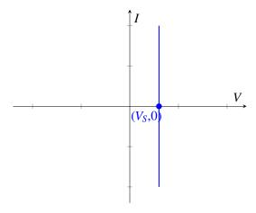
Now if we want to ignore the contribution of this voltage source, we are setting  $V_S = 0$ . Then the I-V plot is exactly the y-axis.
