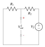
We can see that  $V_{out}^2 = \frac{R_1}{R_1 + R_2} V_2$ . Finally, to get the output voltage  $V_{out}$  of the original circuit, we add the two output voltages based on the response of each voltage source together  $V_{out} = V_{out}^1 + V_{out}^2 = \frac{R_2}{R_1 + R_2} V_1 + \frac{R_1}{R_1 + R_2} V_2$ .
