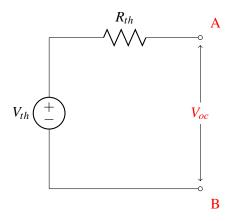
• Intersection with the I-axis: At this point, the voltage across A and B is equal to zero, which is equivalent to shorting A and B. We denote the current at this point be  $I_{sc}$ . Then we know that  $I_{sc} = \frac{V_{th}}{R_{th}}$  by Ohm's law. Hence, we can find  $R_{th}$  by computing  $R_{th} = \frac{V_{th}}{I_{sc}}$ .
