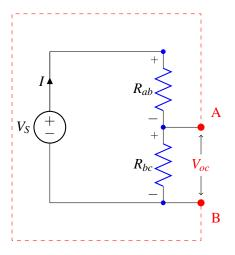
To figure out  $R_{th}$ , we short A and B in the original circuit, find the current  $I_{sc}$  going from A to B, and compute  $R_{th} = \frac{V_{th}}{I_{sc}}$ .
