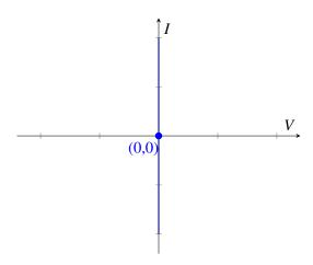
What does this mean? This means that it allows any current to go through, however the voltage drop always remains zero. This is exactly what a short circuit does.
