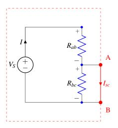
In the specific example we worked with, we can see that  $V_{th} = V_{oc} = \frac{R_{bc}}{R_{ab} + R_{bc}} V_S$  and  $R_{th} = \frac{V_{th}}{I_{sc}} = \frac{\frac{R_{bc}}{R_{ab} + R_{bc}} V_S}{\frac{V_S}{R_{ab}}} = \frac{\frac{R_{ab}R_{bc}}{R_{ab} + R_{bc}}}{\frac{R_{ab}R_{bc}}{R_{ab} + R_{bc}}}$ . So the Thevenin equivalent circuit is
