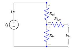
Note that  $R_{bot}$  is the resistor in the bottom plate. We can measure the voltage  $V_{bc}$  to figure out the position at which you touched. Now what if the device you're using to measure the voltage has a resistance R associated with it? Then the circuit becomes
