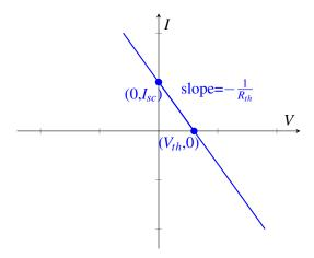
We know once we pin down the values of two points on a line, we can uniquely determine the line. In particular, we look at the following two points
