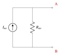
In the Norton equivalent circuit, instead of a voltage source, we have a current source instead. However, the analysis follows very similarly to what we did for Thevenin circuit.
