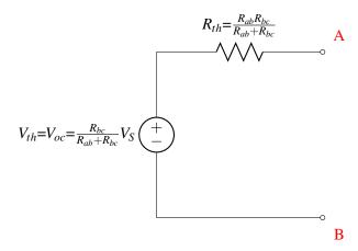
Another way to calculate  $V_{th}$  and  $R_{th}$  is detailed in Section 6.3.3 of Ali Niknejad's Electronics Reader.
