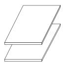
If there is voltage across the two pieces of conductors, charges will build up on the surface of the capacitor. As depicted below, when we apply voltage V across the two plates, positive charges build up on the (bottom) surface of the plate connected to the positive terminal and negative charges build up on the (top) surface of the plate connected to the negative terminal.
