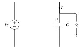
We know that initially, charges are going to build up on the two plates — positive charges on the top plate and negative charges on the bottom plate. Once enough charge has been stored, the voltage across the capacitor becomes  $V_C = V_S$ ; as we will see next, in this next, the current I flowing through the circuit becomes zero.
