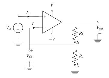
We know that by applying KCL at the junction between  $R_1$  and  $R_2$ , we have
