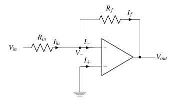
Given an ideal op-amp (with power rails of sufficiently large magnitude), what is  $V_{out}$  if we input an arbitrary voltage of  $V_{in}$ ?
