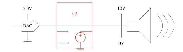
This looks just like the internal of an op amp! Now notice that based on what we know so far about op amps as comparators, we can't just scale the voltage linearly as we we would have wished: if we connect an ideal op amp (infinite internal gain) with  $V_{DD} = 10V$  and  $V_{SS} = 0V$ , the output voltage would either be 10V or 0V, but not something in between. To achieve what we would like, we need another tool, which we will introduce in the next section.
