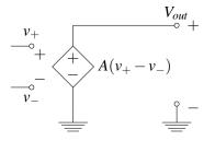
Notice that there is no closed circuit connected to the positive or negtiave input terminal of the op amp. Thus, no current can flow into the positive or negative input terminal. Note that this rule holds regardless of whether there is negative feedback or not.
