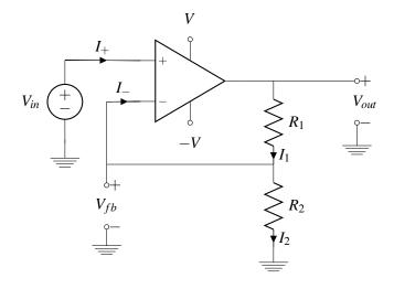
We know that when  $V_{in}$  increases,  $V_{out}$  also increases since  $V_{out} = A(V_{in} - V_{fb})$ . When  $V_{out}$  increases,  $V_{fb} = \frac{R_2}{R_1 + R_2} V_{out}$  also increases, which then cause  $V_{error}$ , and hence,  $V_{out}$  to go down. (Note in this case,  $f = \frac{R_2}{R_1 + R_2}$  in the block diagram.) Now let's derive why  $V_+ = V_-$  in this case. We know that in the above circuit,  $V_+ = V_{in}$  and  $V_- = V_{fb}$ . Let's redraw the block diagram.
