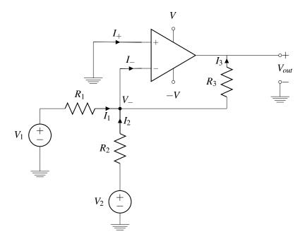
First, let's apply the first golden rule,  $I_{-} = I_{+} = 0$ . Applying KCL at the node labelled  $V_{-}$ , we have
