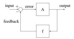
The idea is we take the difference between the input and a scaled version (multiplied by f) of the output, which we call feedback, and apply gain A on it to again produce the output.
