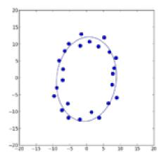
As we can see, the least squares method is useful for fitting known equations to a curve provided that we know the general shape of the curve!
